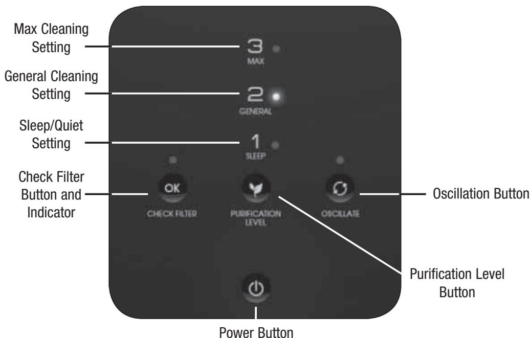
**Check Filters Button** – When it is time to check and clean the filter, an indicator light will illuminate above this button. When this light comes on, you will need to clean your primary ifD® filter and clean or replace your pre-filter. (See Filter Cleaning instructions on page 10). After you have cleaned or replaced the filters, press and hold the Check Filters button for approximately 2 seconds until the light goes off.
